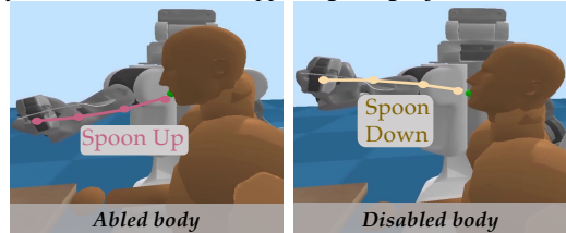
Fig. 8: Assistive Feeding environment. The barrier states represent the horizontal spoon orientation. These states are undesirable for feeding because it misplaces the food in the human’s mouth.
