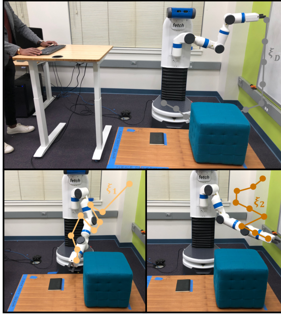
Figure 3.1: Example of a demonstration (top) and a best-of-many choice query with |Q| = 2 , i.e., a pairwise comparison query (bottom). During the demonstration the robot is passive , and the human teleoperates the robot to produce trajectory \xi_D from scratch. By contrast, the preference query can be active : the robot chooses two trajectories \xi_1 and \xi_2 to show to the human, and the human answers by selecting their preferred option.
