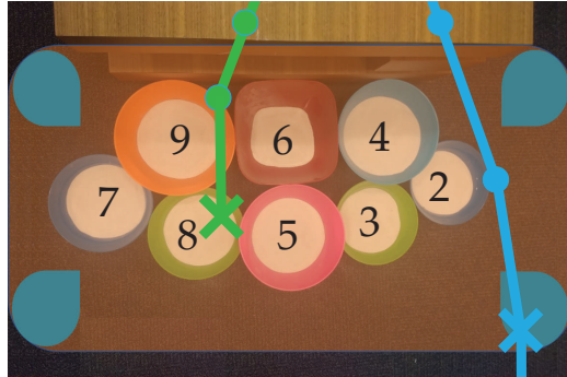
Figure 4.15: Top view of the eight targets in the variant of mini-golf user study. The users assign distinct scores from 2 to 9 to the targets. The figure shows an example of this ranking. While the robot is capable of hitting the ball into the entire shaded region, the maximizers of a linear reward always lie near the corners of the shaded region in blue. Therefore, while the GP reward model can query the user with better trajectories (e.g. the green trajectory), the linear model only explores the boundaries (e.g. the blue trajectory that throws the ball outside of this region). Crosses show where the ball hits the ground.
