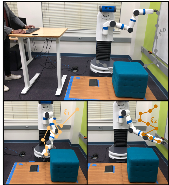
Figure 2. Example of a demonstration (top) and preference query (bottom). During the demonstration the robot is passive , and the human teleoperates the robot to produce trajectory \xi^D from scratch. By contrast, the preference query is active : the robot chooses two trajectories \xi_1 and \xi_2 to show to the human, and the human answers by selecting their preferred option.
